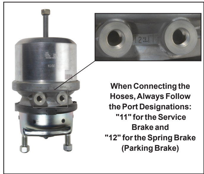
Figure 12 – Bendix® Piston-Style Spring Brake Port Connections
