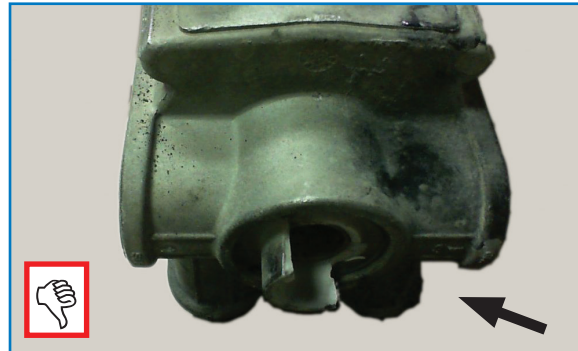
Example of a Bendix® QR-1® Quick Release Valve with a damaged port due to an external impact.
